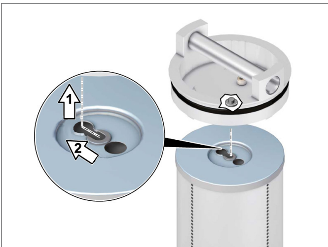
Fig. 9: Attaching the filter element
