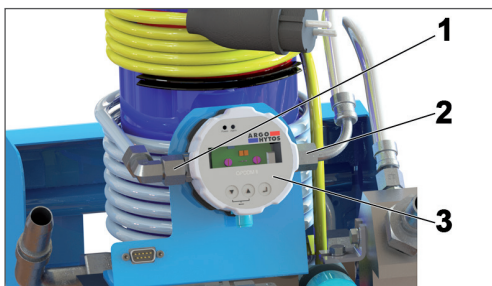
Fig. 13: Replacing the measuring sensor
