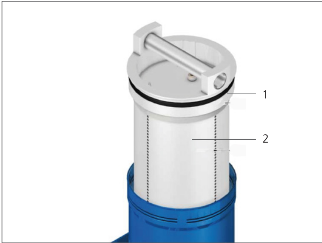
Fig. 10: Installing the filter element
