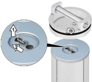
Fig. 7: Attaching the filter element
