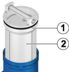
Fig. 5: Removing the filter element
