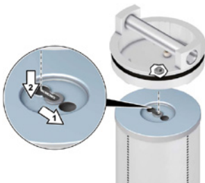
Fig. 6: Removing the filter element from the cover
