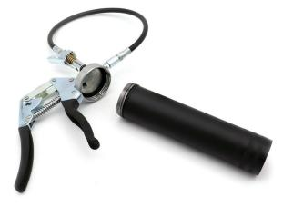
Remove the bottom cover from the cartridge of grease (typically a plastic cap)
