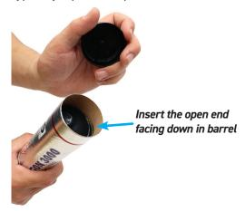
Insert the open end of the grease cartridge first
