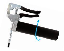
Begin pumping until grease starts to flow out of the coupler
