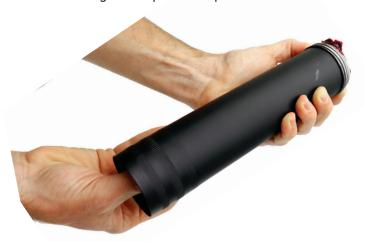
Screw the head of the grease gun back onto the barrel loosely
