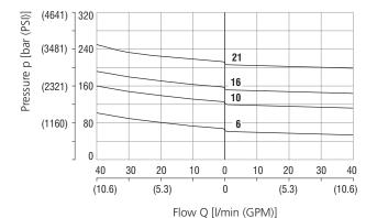
Pressure drop related to flow rate Flow direction P-A Fully open valve through section
